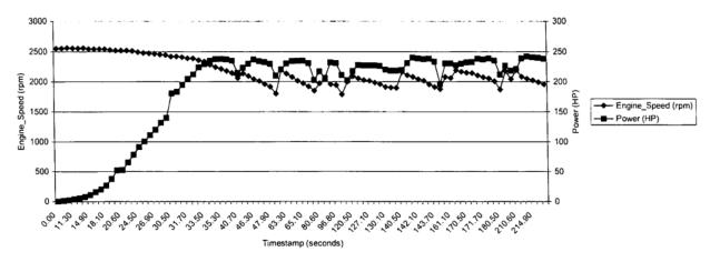
Figure 3-6. Before Mileage Accumulation Horsepower Test Results #2
