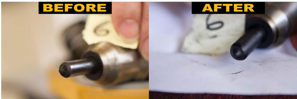
Figure 3-3. Before and After Pictures of Fuel Injectors.
